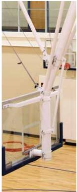
Provides great stability at tall heights, the TF-20S Basketball Backstop's bent stem reduces space between pivot point and jackknife to assist in avoiding obstructions. Backstops are custom designed so the lateral sway brace intersects the main mast at approximately 54" (1.37 m) above the goal and 18" (45.7 cm) above the backboard to ensure maximum rigidity.
